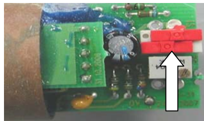
Pic. 8: Delay switch version from serial no. <436
