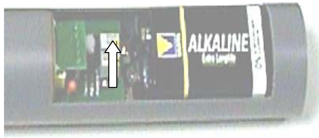
Pic. 7 Delay adjuster version until serial no 436
