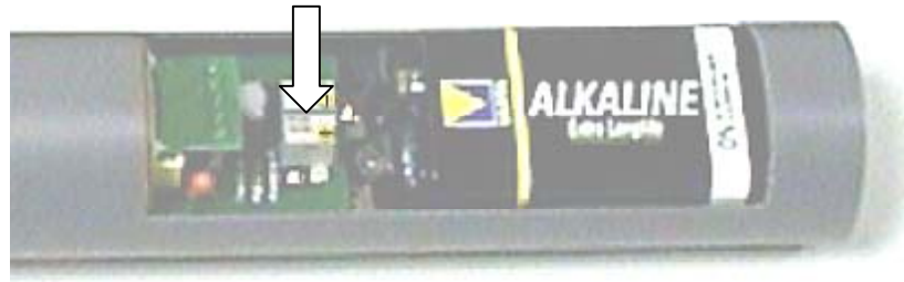
Pic. 7: coarse adjuster for sensitivity inside battery compartment
